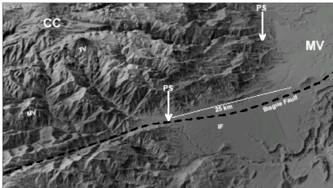
Figure 2. Physiographic shaded relief map based on STRM data of 30 m resolution. Note the tilted planation surface remnants in the east flank of the Central Cordillera (CC) and their right lateral displacement by the Ibagué Fault. Magdalena Valley (MV), Planation Surface (PS), Ibagué Fan (IF), Volcano Machín (VM) and Volcano Tolima (VT).
